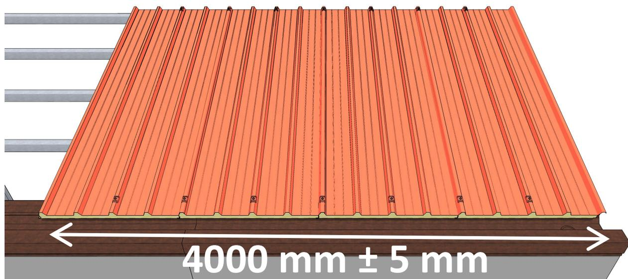
**Note:** take care to properly place the panels during the assembly step (4 panels = 4000 mm ± 5 mm) in order to prevent problems during the next ridge installation step, as shown in the figure.
