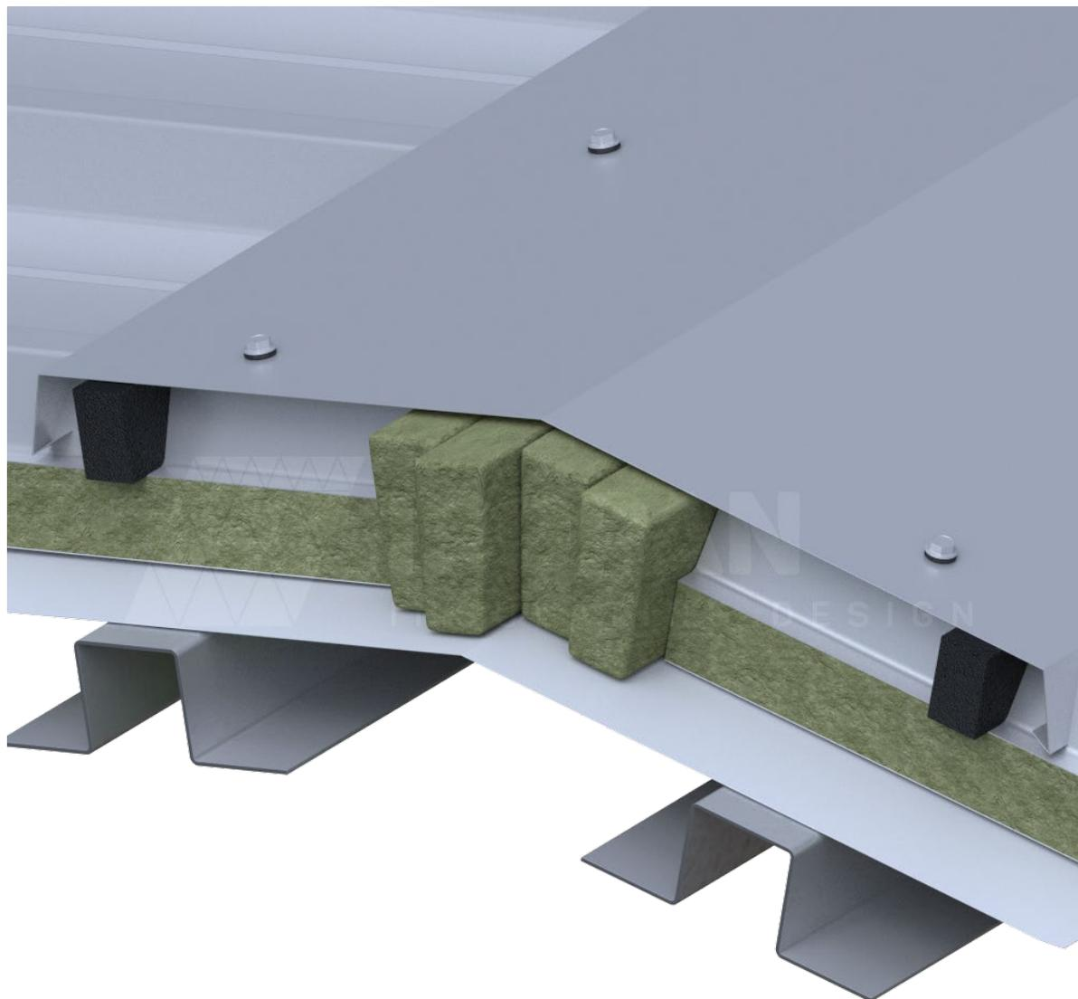
Type 1 roof ridge: vertical cross-section
