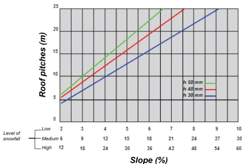
In the former case, the minimum slope, in relation to the climatic area and the rib height, can be taken from the **Slope diagram**. We recommend (in the event of low or average level of snowfall) a slope no less than 7%.
