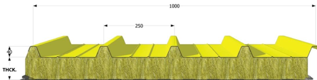
Self-supporting, double skin sandwich panel for roofing with 5 ribs, featuring a mineral fibre core that assures excellent thermal insulation. It was developed to meet growing performance needs on sound absorption and sound insulation behaviour, keeping high mechanical and insulation characteristics.
