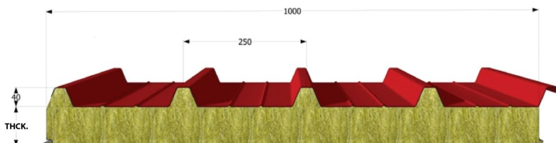
Self-supporting, double skin sandwich panel for roofing with 5 ribs, featuring a mineral fibre core that assures the product's incombustibility in addition to assuring excellent thermal insulation. It was developed to meet growing performance needs and legislative constraints on fire behaviour for buildings, keeping high mechanical and insulation characteristics.
