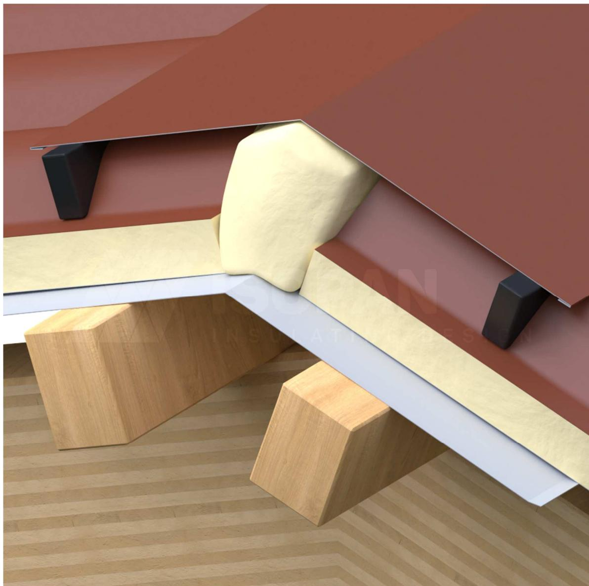
Type 5 roof ridge: vertical cross-section
