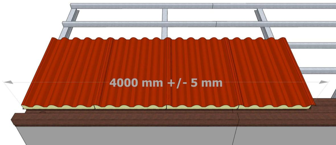
**Note: take care to properly place the panels during the assembly step (4 panels = 4000 mm ± 5 mm) in order to prevent problems during the next ridge installation step, as shown in the figure.**
