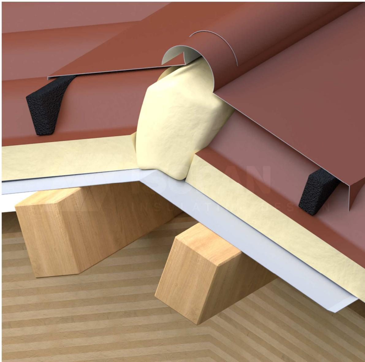
Type 6 roof ridge: vertical cross-section
