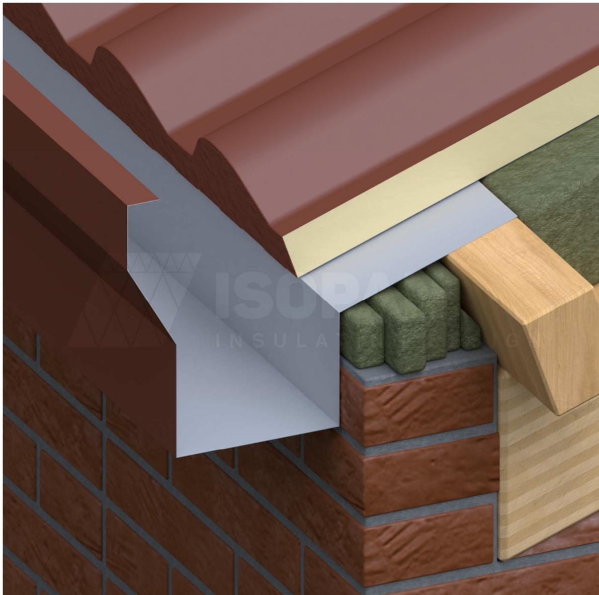
Detail of gutter side on traditional structure - with liquid sheath
