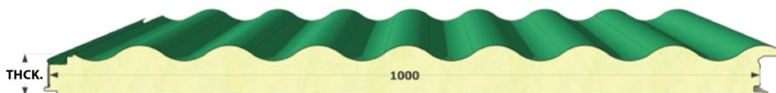
Double skin metal faced wall sandwich panel with polyurethane foam insulating core, used to build curtain walls in civil and industrial buildings, featuring a tongue-and-groove concealed joint system that makes for long-lasting and sleek constructions. The corrugated profile offers a high aesthetic and architectural value.
