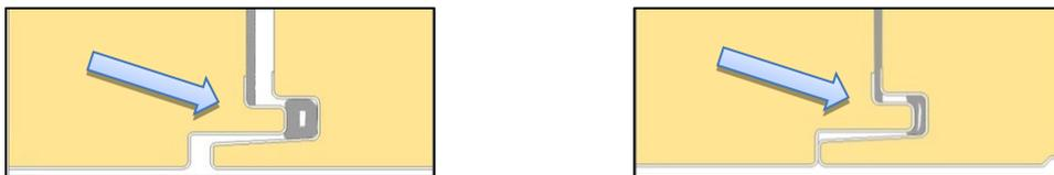
Gasket crushing, leading to increased seal, due to the side pressure required to assure suitable coupling
