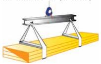
Suitable spacers must be used consisting of robust lengths of flat timber or plastic located above and below the pack, in order to prevent direct contact between the slings and the pack.
