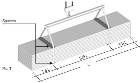
Suitable spacers should be positioned above and below the package. These should be flat wooden or plastic elements that prevent direct contact between the belt and the package. They must be at least 4 cm longer than the package and at least as wide as the belt.
